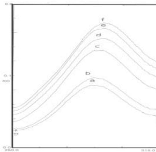
**Fig: 1** U.V. Spectra of solubilised iodine ( $\lambda_{max} = 289.95$ ) in Tween 80 solution with different concentration. a = 0.0008 mM, b = 0.0009 mM, c = 0.001 mM, d = 0.0015 mM, e = 0.002 mM, f = 0.003 mM.
