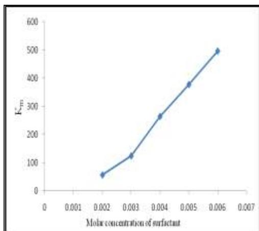
**Fig: 8** Graph between the Micelle water partition coefficient ( $K_m$ ) verses molar Concentration of Brij 35.
