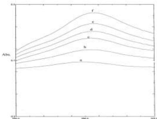
**Fig: 3** U.V. Spectra of solubilised iodine ( $\lambda_{max}$ = 289.95) in brij 35 solution with different concentration. a = 0.0008 mM, b = 0.0009 mM, c = 0.001 mM, d = 0.0015 mM, e = 0.002 mM, f = 0.003 mM, g = 0.004 mM.
